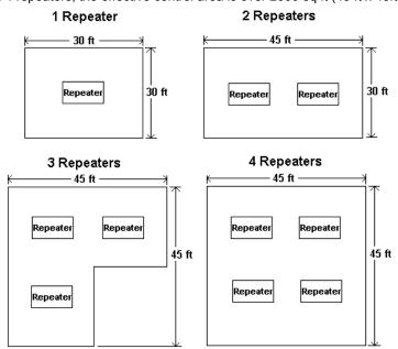
Recommended placement for 1-4 Repeaters. Note: The distance between repeaters or the edge of your model railroad layout is recommended to be 15ft or less.
