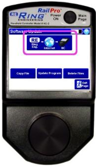
5) When a new program for the handheld controller is finished downloading, the screen will display updating now please wait xx seconds. Then the handheld controller will start up and the new program will be loaded.
