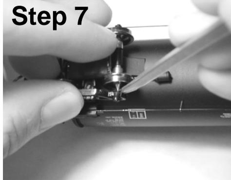
Use 1/8 inch Flat Blade Screw Driver and gently pry each side frame out just far enough to re-insert the axle into the side frame pockets. See caution from Step 2.
