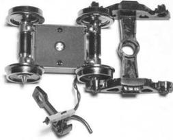
The circuit board can now be flipped out of the way to expose the mounting screw hole.
