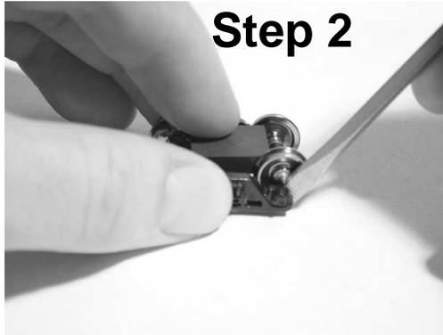
Use 1/8 inch Flat Blade Screw Driver and free axle farthest from EOT. **Important:** See next picture. Gently, pry each side frame out just far enough to free the axle from the side frame pocket.
