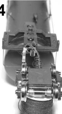
Support Truck assembly and install coupler to train car.
