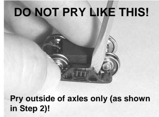
Pry outside of axles only (as shown in Step 2)!
