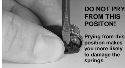
**CAUTION:** The axles are attached to the circuit board by a light gauge wire that can be damaged if care is not taken during this step and step 4. Physical damage will be considered abuse and will not be covered under the limited warranty!
