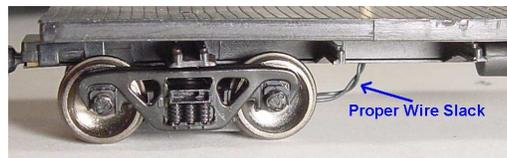
Set the wire slack so the truck can rotate enough to accommodate your tightest radius turn but be sure the wire does not hang down below the railhead of the track. Once the wire slack is correct, put some white glue or silicon sealant in the hole the wires pass through to hold their position. Do not use glue that will dissolve the insulation on the wire.
