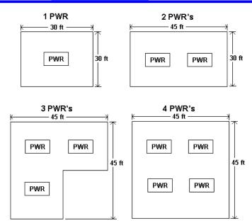
Recommended placement for 1-4 PWR's. Note: the distance between PWRs and the edge of your model railroad layout should be 15 ft or less.
