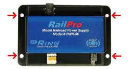
The only acceptable mounting orientations are: 1) Mounted to the bottom surface of the layout with the RailPro logo facing the ground or 2) Set on top to the layout with the RailPro logo facing the roof. Also there should be at least 2 inches of space on each side for air circulation.
