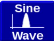
This creates a sine shape of sample brightness based on the length of samples that you enter. The index must be set before this tool is used because the first sample starts at the current index. If you set the index to sample 0 and then use the Sine Tool with a value of 56 then the sample will start in index 0 and will draw a sine shape over a time of one second. Things like ditch lights can oscillate in a sine pattern.
